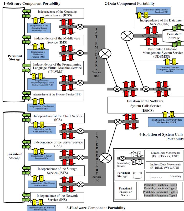
Fig. 11. COSMIC-SOA reference architectural model of system portability requirement.
