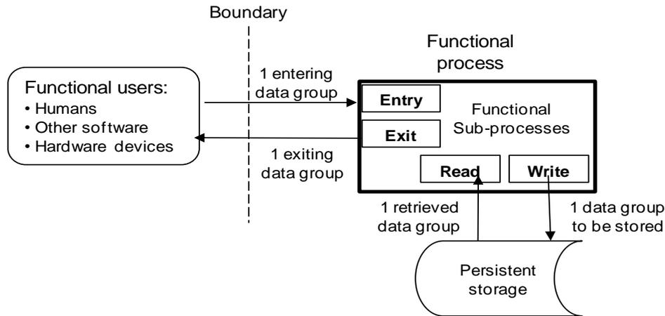
**Figure 3.5 – The four types of data movement, each moving one data group, and their relationship with a functional process. (A functional process can, of course have many E, X, R and W data movements.)**
