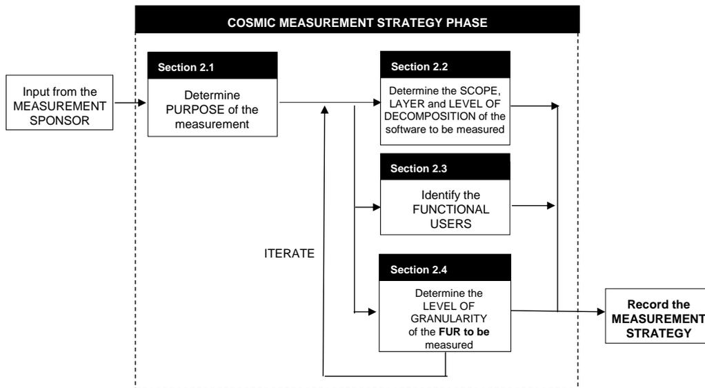
**Figure 2.0 - The process of determining a Measurement Strategy**
