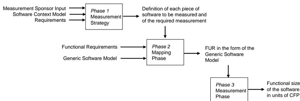
**Figure 1.4 – The COSMIC method measurement process**
