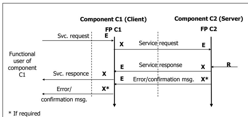
**Figure 3.7 – Data exchanges between client and server components**
